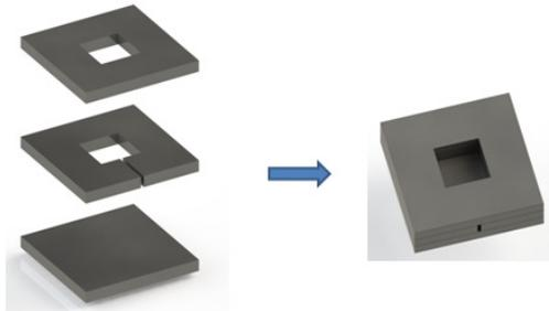
Fig. 4. The virtual assembly of the enclosure
