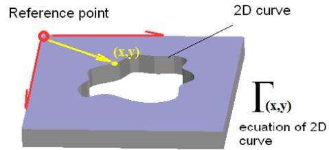
**Fig. 2. A cavity obtained by cutting of sheet**
