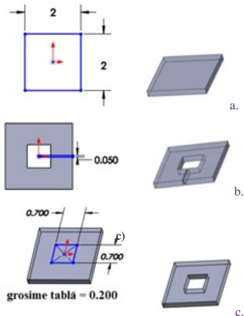
**Fig. 3. The design for enclosure layers**
