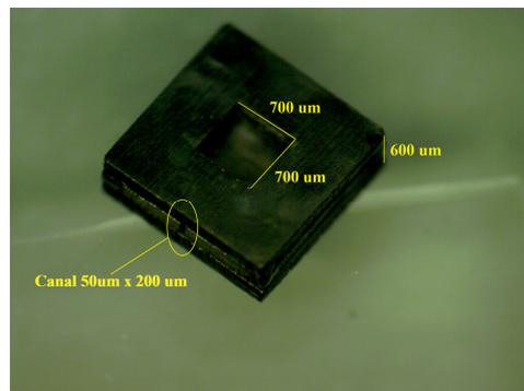
Fig. 8. The microlitric enclosure
