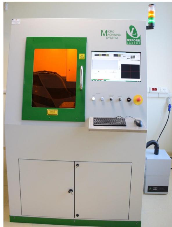
Fig. 1. Laser ablation system
