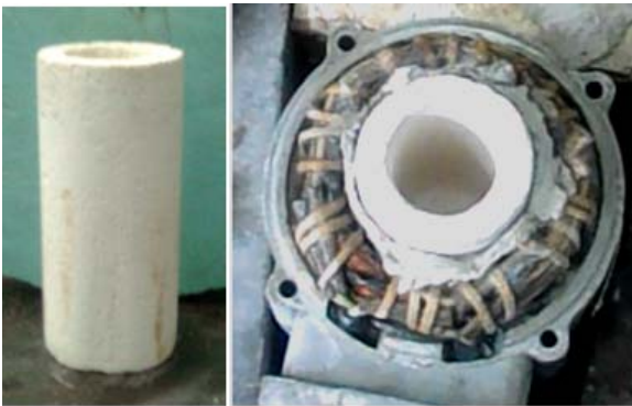
Fig.2. Casting mould of refractory material and way of place in rotating electrical field generator
