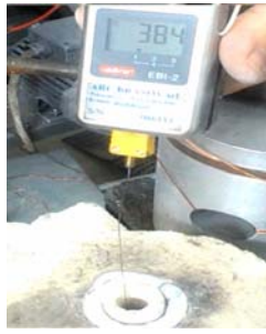
Fig.9. The temperature of ZnAl4Cu1 melt under the action of rotating electric field
