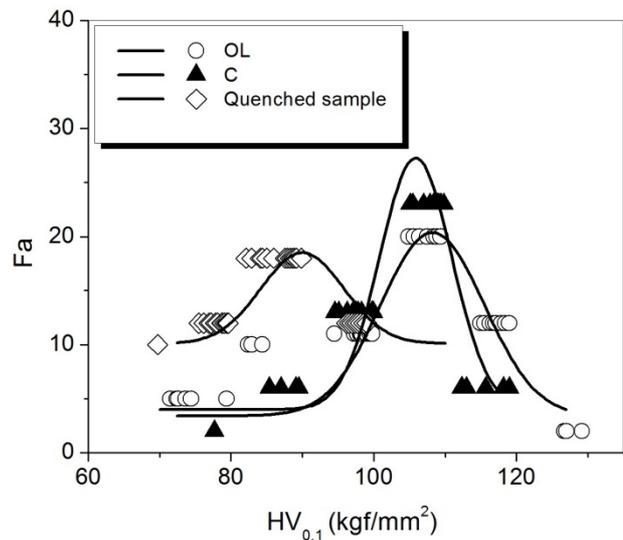
Fig. 6. Frequency distribution function to  $HV_{0.1}$  for s.s. $\alpha$  and s.s. $\beta$  of Zn-22 wt % Al alloy obtained in different processing conditions
