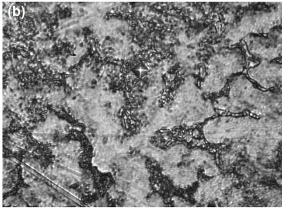
Fig. 3. Indentations on phase and constituent of the cast Zn-22 wt % Al alloy in steel moulds: (a)  $\alpha$ ; (b) eutectic ( $\alpha + \eta$ )
