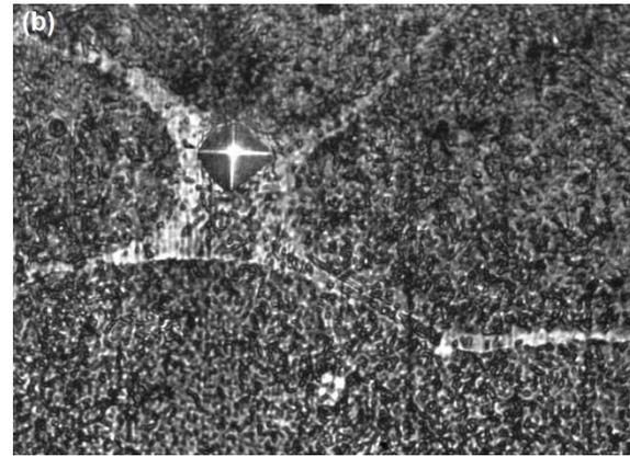
Fig. 5. Indentations on phase and constituent of the quenched Zn-22 wt % Al alloy: (a)  $\beta$ ; (b) eutectic ( $\alpha + \eta$ )
