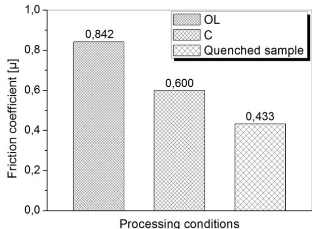
Fig. 10. Coefficient of friction versus processing conditions for Zn-22 wt % Al alloy
