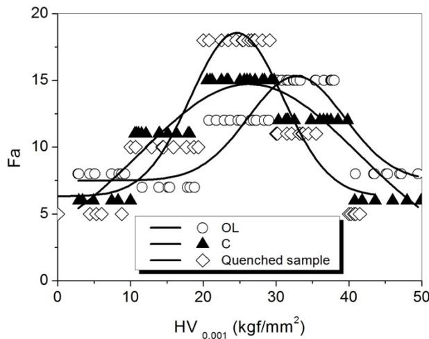
Fig. 8. Frequency distribution function to  $HV_{0.001}$  for interdendritic eutectic ( $\alpha + \eta$ ) of Zn-22 wt.% Al alloy obtained in different processing conditions
