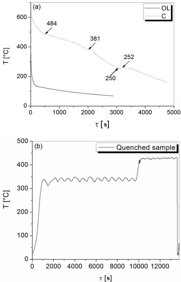
**Fig. 1. (a) Cooling curves for Zn-22 wt % Al alloy cast in various moulds; (b) Heating – maintaining-cooling curve for quenched sample**
