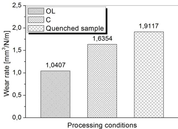
Fig. 11. Wear rate versus processing conditions Zn-22 wt % Al alloy
