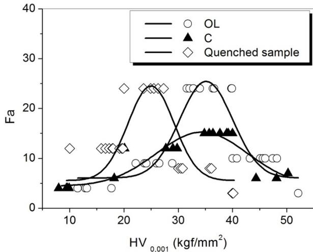
Fig. 7. Frequency distribution function to  $HV_{0.001}$  for s.s. $\alpha$  and s.s. $\beta$  of Zn-22 wt % Al alloy obtained in different processing conditions
