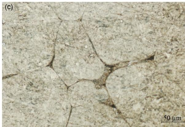
**Fig. 2. Microstructure of the cast Zn-22 wt % Al alloy: (a) in steel moulds; (b) in brick moulds; (c) quenched**
