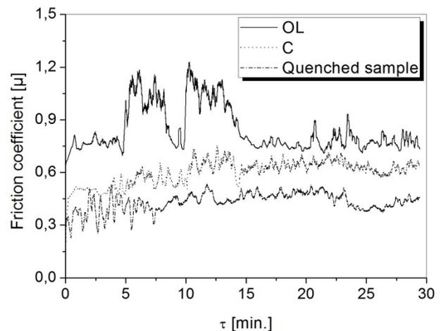
Fig. 9. Coefficient of friction versus time for Zn-22 wt % Al alloy
