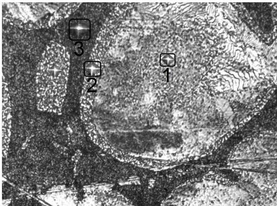
Fig. 4. Indentation on phase and constituents of the cast Zn-22 wt % Al alloy in brick moulds: 1 -  $\alpha$ , 2 - inter-dendritic spacing ( $\alpha + \eta$ ), 3 - eutectic
