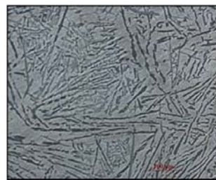
Fig. 3. Microstructure of sand casting sample
