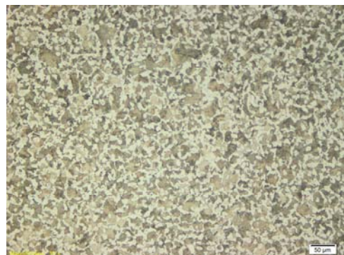
Fig.1 The specific structure of rolled metal (ferrite-pearlite structure) for C45E Magnification (X200). Attack Nital 5%
