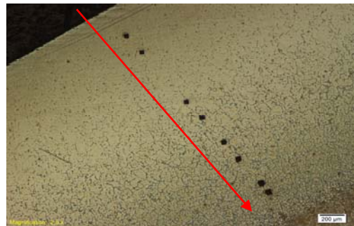
Fig. 5 Measuring the induction hardened coating microhardness and depth of Magnification (X50)
