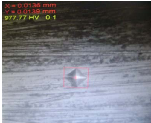
Fig. 7 Measurement of microhardness on the outside surface of C45E chrome bar Magnification (X200)
