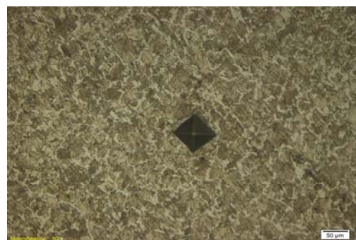
Fig.2 Measurement of microhardness in the steel C45E. Magnification X 200 Attack Nital 5%.
