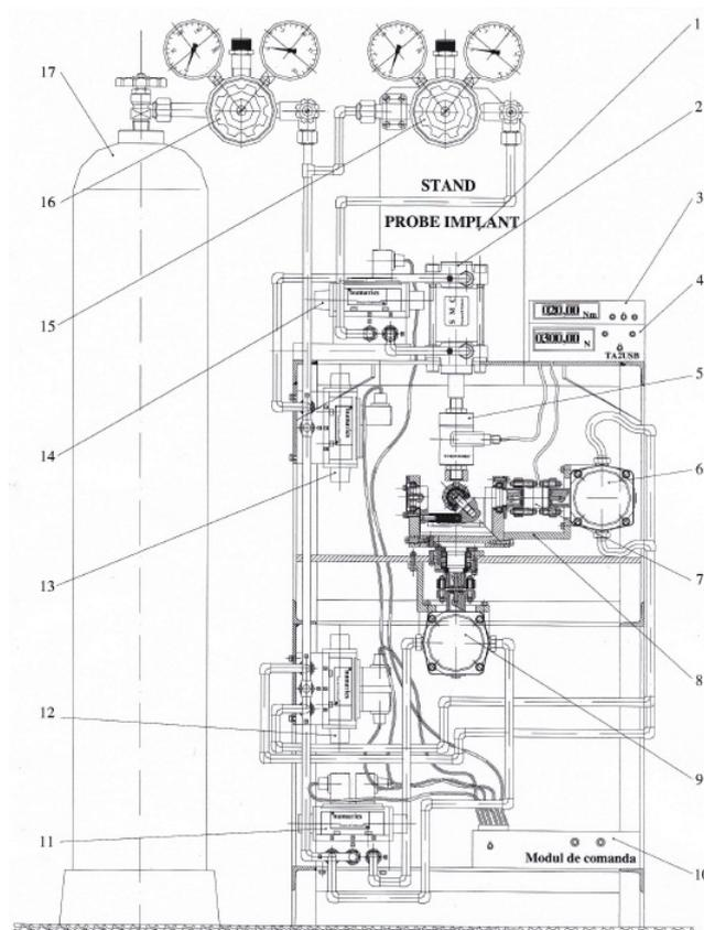
Figure 8. Experimental stand for testing the friction torque on the femoral head of a hip prosthesis
