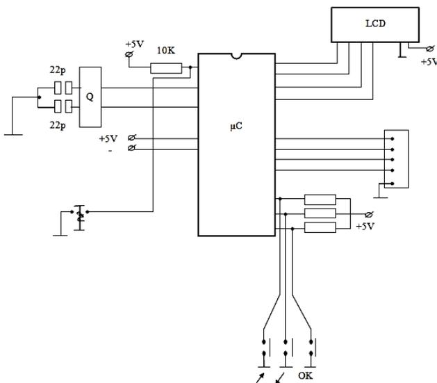
Figure 13. The electronic diagram of the control unit
