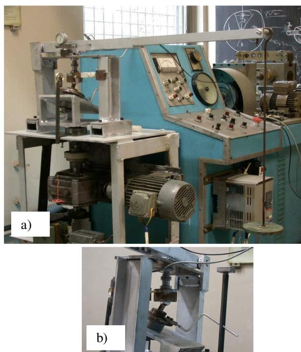
**Figure 3. Experimental stand for tribological study of hip prostheses, made at the Department of Machine Elements and Tribology, University Politehnica of Bucharest [6]. a) overview, b) detail**
