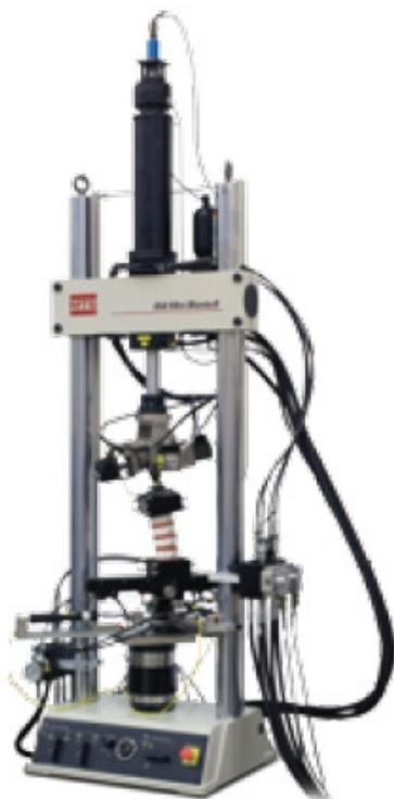
Figure 7. Professional system for dynamic multiaxial testing
