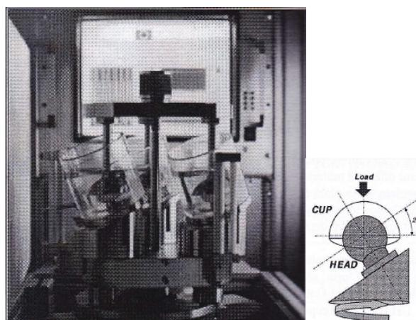
**Figure 4. HJS simulator with three operating positions [7].**
