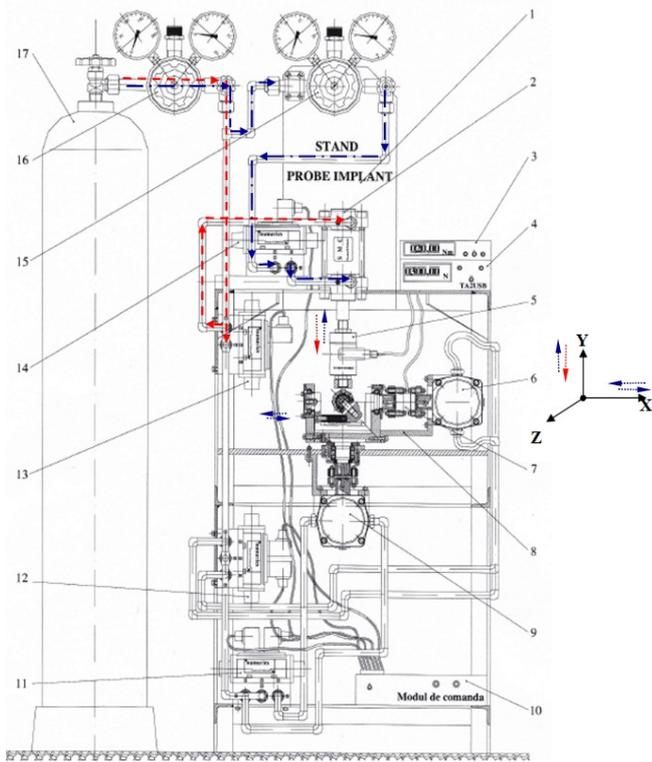
**Figure 9. The circuit of the fluid used for the translation movement on the Y axis**
