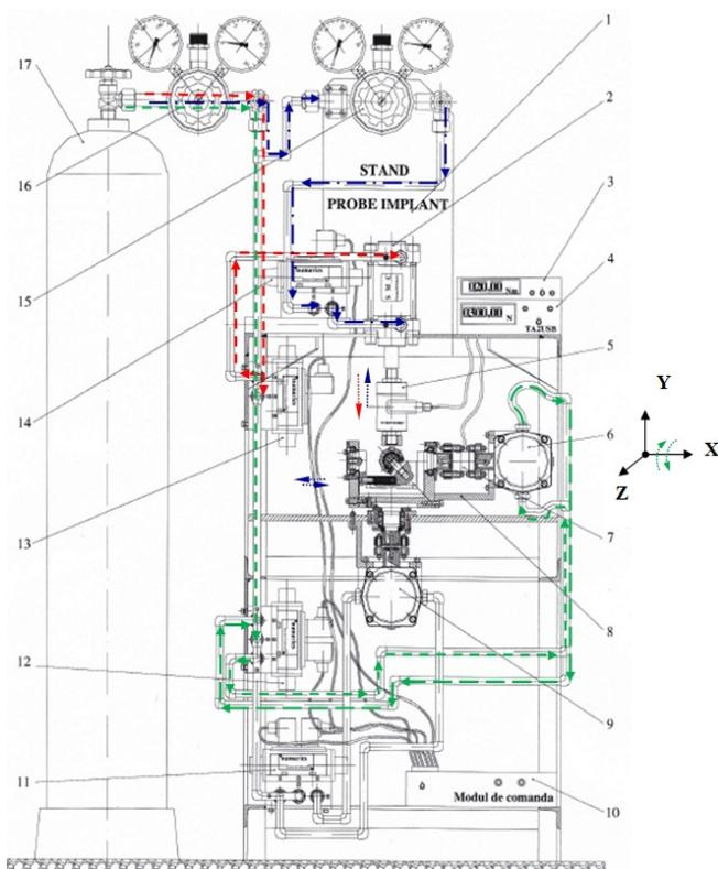
**Figure 10. The circuit of the fluid used for the flexion-extension movement**
