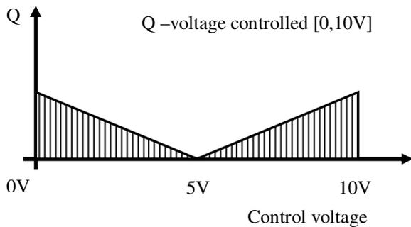
Figure 12. Control feature of the electro-distributors
