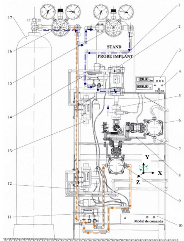
**Figure 11. The circuit of the fluid used for the internal rotation-external rotation movement**
