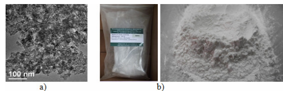
Figure 1. a) TEM image of Al_2O_3 nanoparticles; b) Al_2O_3 nanoparticles, 10nm size
