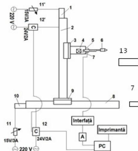
Figure 1. Scheme of the mechatronic system experimental model
