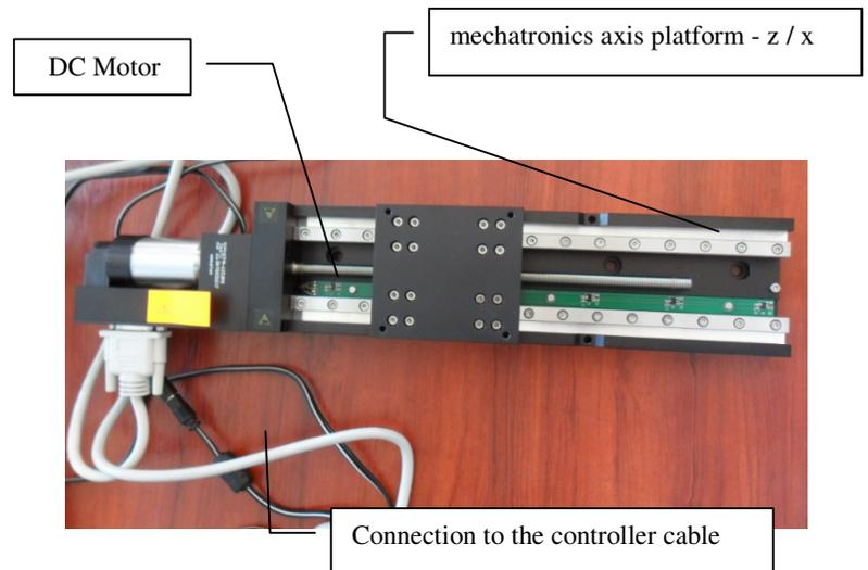
**Figure 11. Electric linear axis**
