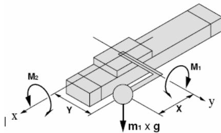
**Figure 4. Mechatronic axis x horizontal assembly**
