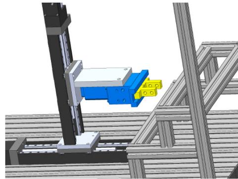
**Figure 6. Highlighting the x and z axes and location of the microgripper bracket**
