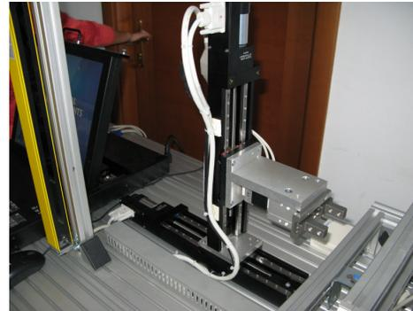
**Figure 10. Positioning system, consisting of two vertically-mounted linear axis**
