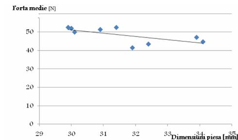
Figura 16. The linear evolution of the clamping force depending on the size of the workpiece
