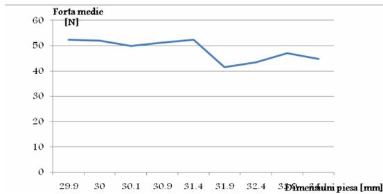
Figure 15. Trend of variation of average clamping force depending on the size of the workpiece
