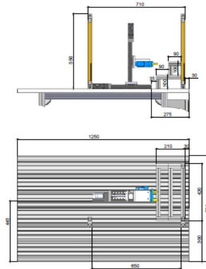
**Figure 5. Representation of the placement of the linear axes and pieces magazine**
