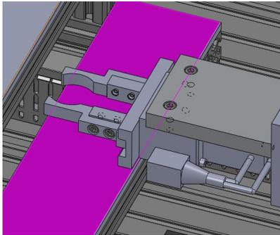
**Figure 7. Representation of the gripper from micro-mechatronic flexible positioning system**
