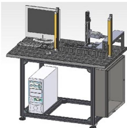
**Figure 9. Representation of the whole micro-mechatronics flexible positioning system**
