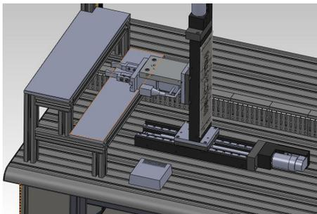
**Figure 8. Representation of linear axes x and z and gripper**
