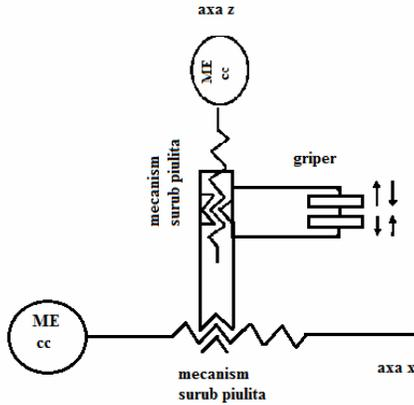
**Figure 2. Kinematic scheme of mechatronic micro-positioning system**
