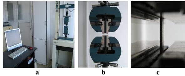
**Fig.3. Hounsfield-H10KT test machine (a) sample holder (b), the sample detail (c)**
