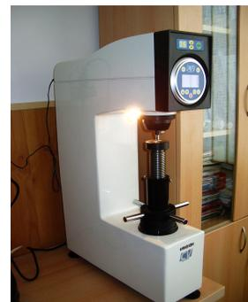
Fig.2. Rockwell hardness tester type NAMICON
