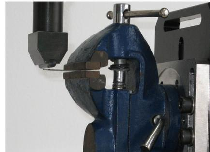
Fig.8. Sample holder of cantilever beam and application system of bending force
