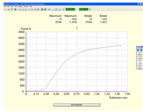
**Fig.5. Traction test graph for CoCrMo sample (sample length 25 mm)**
