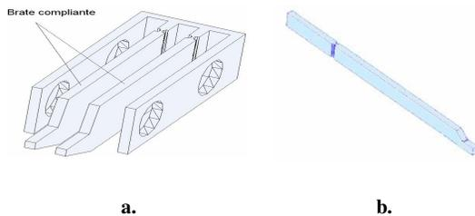
Fig.1. Device assembly (a) and actuator arm (b)
