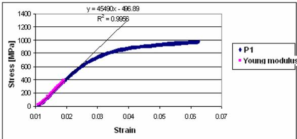
Fig.6. Stress-strain curve for CoCrMo sample
