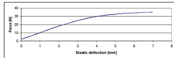
Fig.9. Elastic deflection specimen vs. applied force
