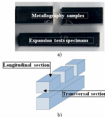
**Figure 1. a) - Gauge block section for metallography and expansion test; b) - drawing for metallography samples in longitudinal and transversal section**
