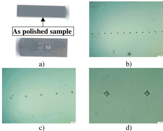
Figure 4. a) – Sample for microhardness indentation; b, c, d) – Indented sample
