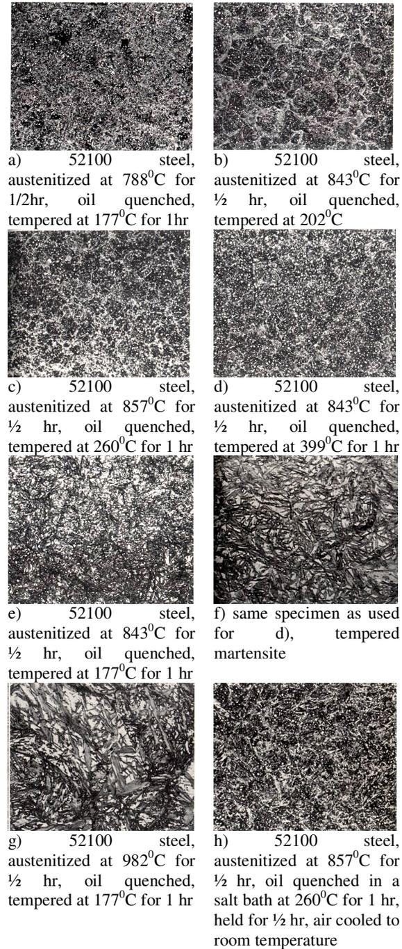
**Figure 2. Microstructures of 52100 steels from Metal Handbook [2]**
