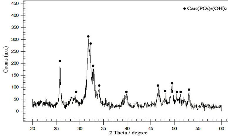
**Fig. 1. X-ray diffraction spectrum of the synthesized hydroxyapatite powders heat treated at 200°C**
