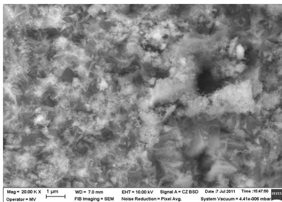
**Fig. 4.** SEM micrographs for hydroxyapatite powders heat treated at 200°C
