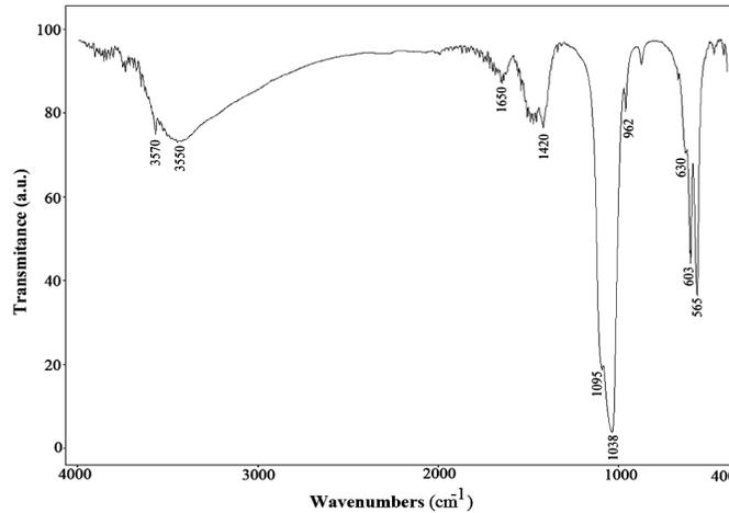
Fig. 2. FTIR spectra of synthesized hydroxyapatite powders heat-treated at 200 °C
