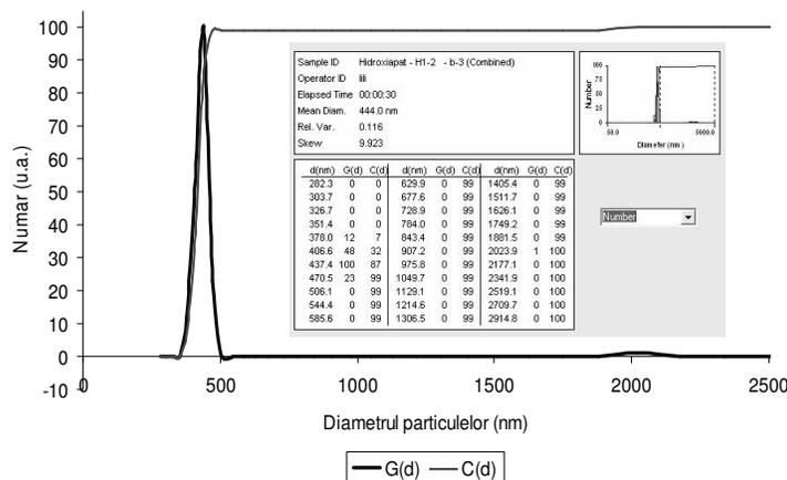
Fig. 3. Particle size distribution of hydroxyapatite powders heat-treated at 200 °C
