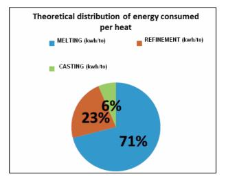
Reduction of development (reduction of melting time) in phase 1, requires the implementation of an additional melting using chemical energy (gas and oxygen). Reducing the amount of electricity consumed by 30% means introducing a flame burner with a maximum output of 1.2 MWh / batch.
