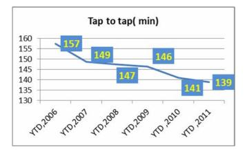
If in the first year of operation the gain was 40 kWh / t and 8 minutes per batch, using control techniques stataistic Phase 2, the 18 minutes decreased concomitantly with a decrease in total energy consumption by 27 kWh / t.
