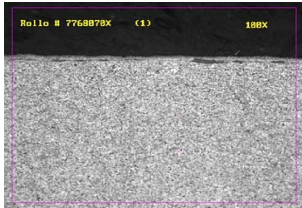
Figure 12. Metallographic examination of etched specimens (E coil; x100)
