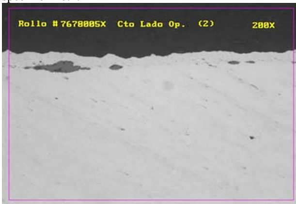
Figure 5. Metallographic examination of un-etched specimens (C coil)
