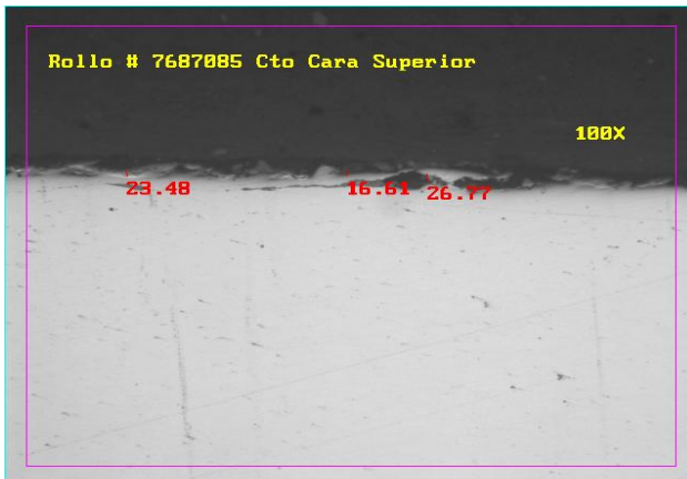
Figure 2. Metallographic examination of un-etched specimens (A coil)
