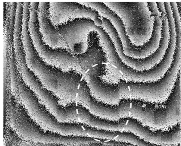
Figure 12. Wrapped, full displacement map of the populated board fixed in the 5 corners, seen from the components side
