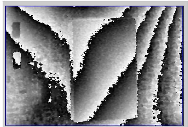
Figure 16. Detailed interferogram showing the fringe pattern on and around the PQFP under thermal stress
