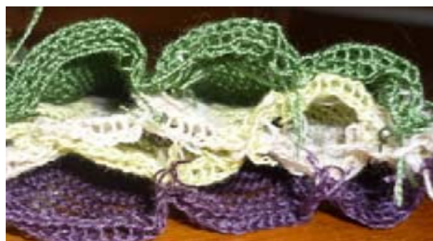
Figure 2 - Cross section of the direction of rows in knit sandwich
