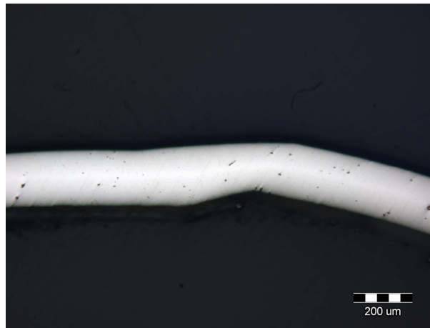
Figure 5: Weld seam, magnification 100x, without metallographic attack.
