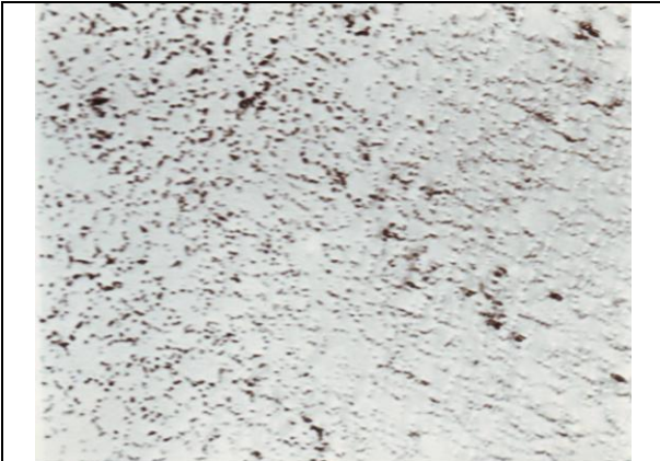
Figure 2. Microstructure of a Y 25 sample (1050 0 C hardening heat treatment, 1h, water and sensitize 600 0 C, 30h, after testing with sulfo cupric solution) Chromic anhydride attack, magnification x250
