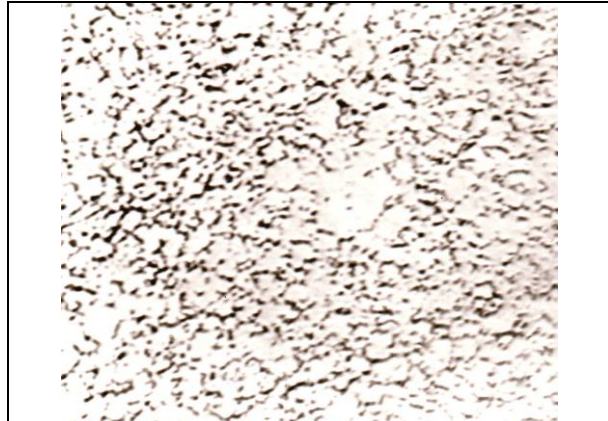
Figure 5. Microstructure of a Y 29 sample (1058 0 C hardening heat treatment, 1h, water and sensitize 650 0 C, 100h, after testing with sulfo cupric solution) Chromic anhydride attack, magnification x250
