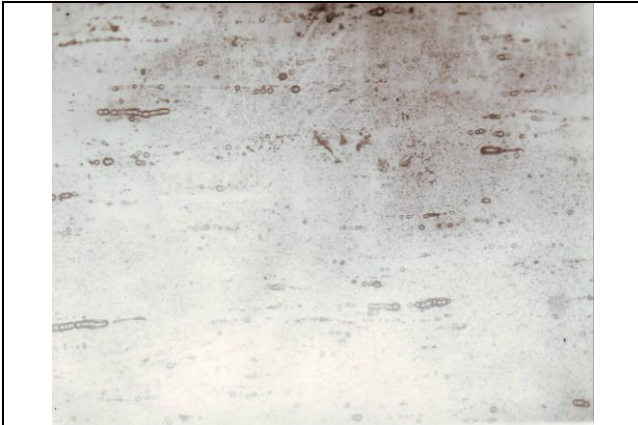
Figure 8. Microstructure of a Y29 sample after testing nitric acid solution, 240 h heat treatment hardening 1050°C, 1 h, water, Chromic anhydride attack, magnification x250
