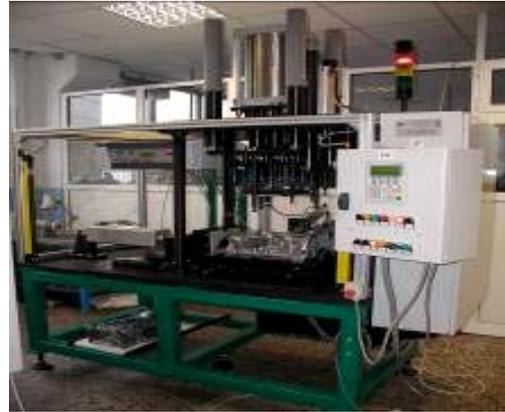
**Fig. 18. Intelligent mechatronic technology and equipment for oil carter tightness control**
