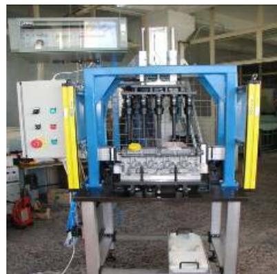
**Fig. 19. Intelligent mechatronic technology and equipment of tightness control for assembled cylinder head of F8Q engine**
