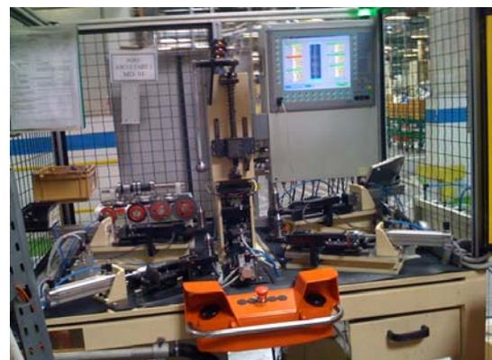
Fig. 12. Intelligent Mechatronic Technology and equipment for controlling uniformity of auto gearbox gears by means of forced engagement (double flank)
