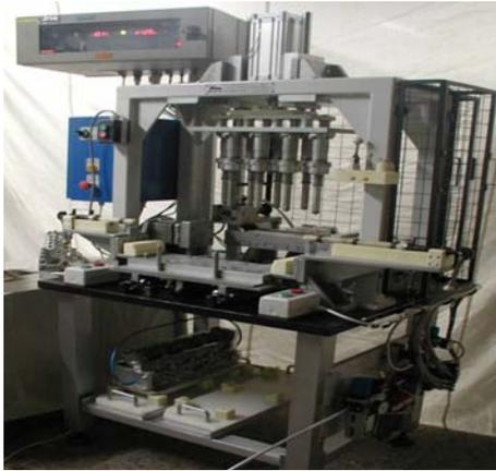
**Fig. 16. Equipment for tightness control of cylinder head and marking**
