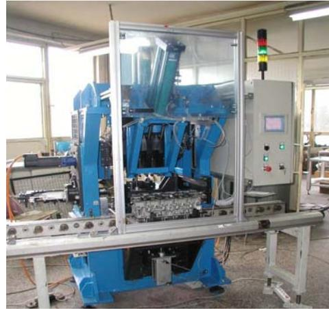
Fig. 11. Tappets controlling and sorting machine with dynamic mobile
