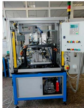
**Fig. 15. Tightness control intelligent mechatronic equipment (in vacuum) for gear carter JH3**
