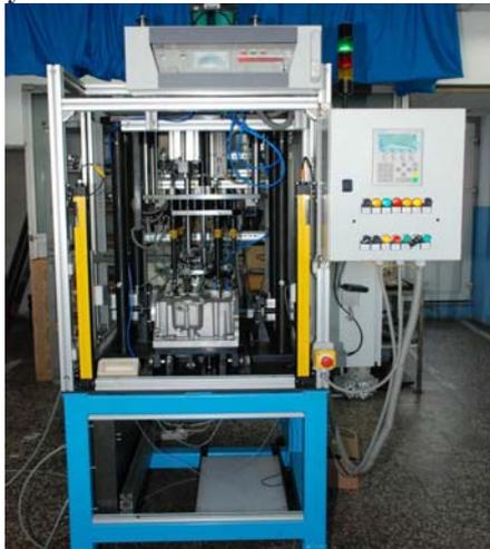
**Fig. 17. Intelligent mechatronic equipment for measuring the tightness of the cylinder carter assembly**
