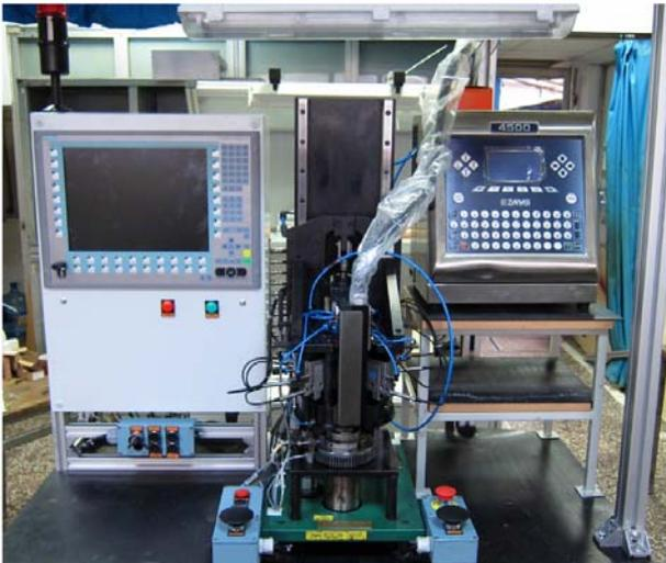
Fig. 6. Mechatronic equipment for geometric control and marking of drum parts
