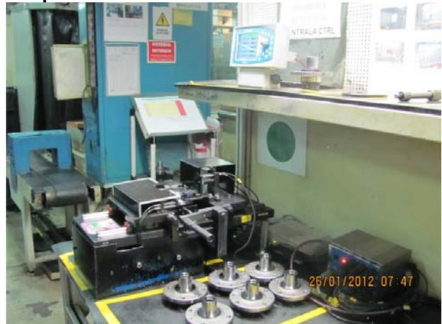
Fig. 7. Mechatronic equipment for geometric control of hub parts
