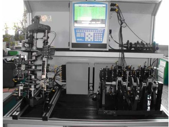
Fig. 8. Mechatronic control equipment for crankshafts
