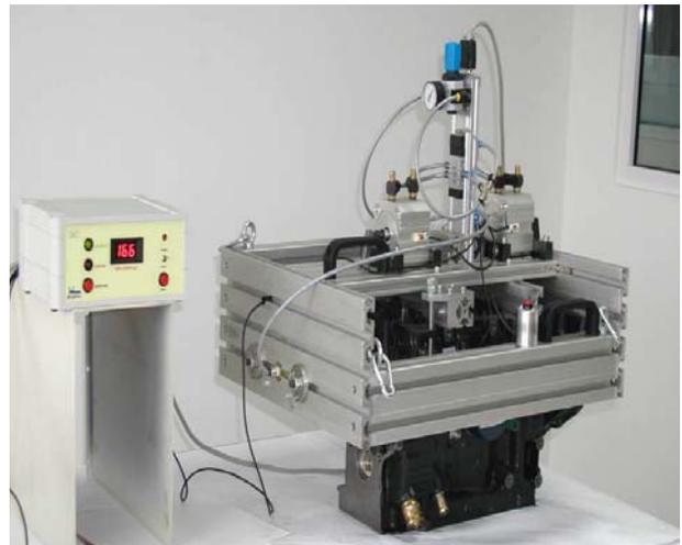
Fig. 4. Equipment for engine control parameters: load torque, axial clearance and presence bearings
