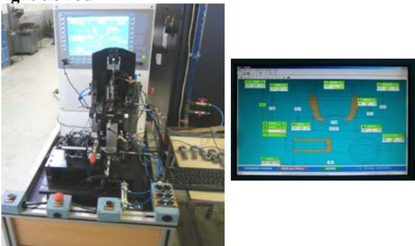
Fig. 10. Mechatronic equipment to control the left and right tie rod
