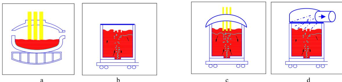
**Fig. 1. The process of developing and refining steels**
