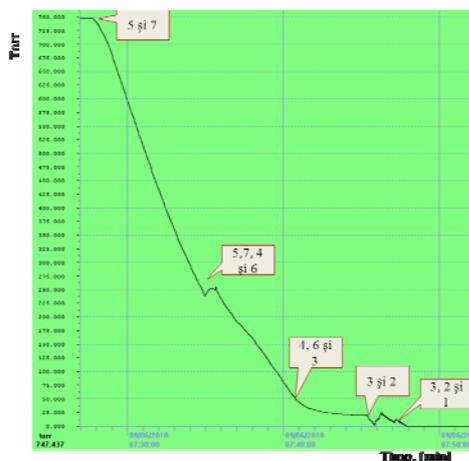
Fig. 4. Coupling vacuum ejectors and time
