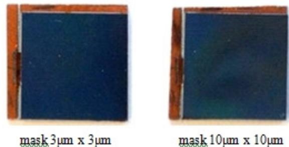
Fig. 6. Micro processed solar cells (2cm x 2cm)
