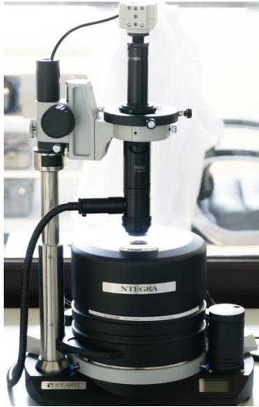
Fig. 7. NTEGRA Prima atomic force microscope
