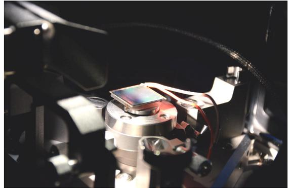
Fig. 9. Preliminary alignment of the sample for the AFM investigations
