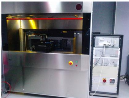
Fig. 3. DWL 66fs system used for making the masks
