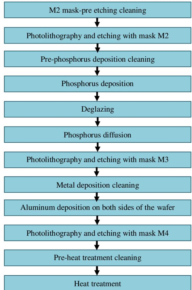
Fig. 5. The process flow used in the manufacturing of mono-Si solar cells by surface micro structuring
