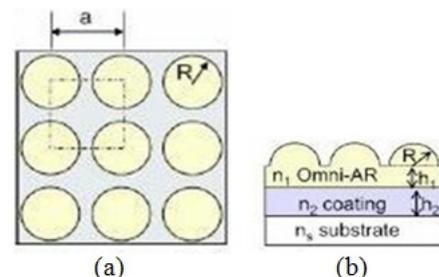
Fig. 2. The structure of an antireflection coating AR a) top view of the AR coating surface, b) longitudinal section of the AR coating [3]
