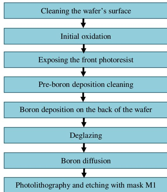
Fig. 4. Flow chart for the front surface micro processing
