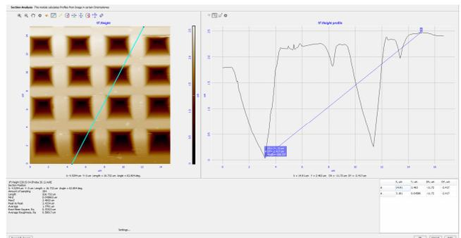
**Fig. 11. Determining the micro processing depth for the sample obtained with the M1 (3µm x 3µm) mask**
