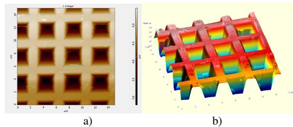
Fig. 10. AFM topography after processing with the M1 ( $3\mu\text{m} \times 3\mu\text{m}$ ) mask
