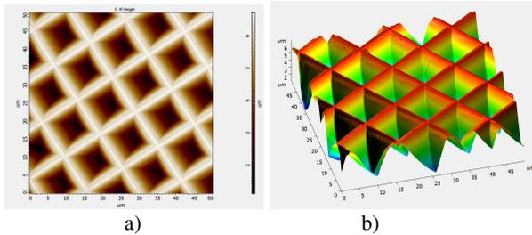
**Fig. 12. The AFM topography after processing with the M2 (10µm x 10µm) mask**
