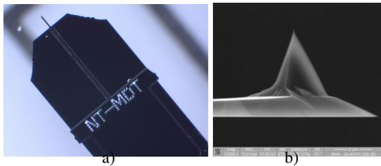
Fig. 8. CSG10 / 10 Cantilever used for the AFM investigations
