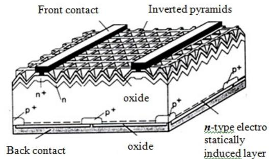
Fig. 1. Structure of a surface micro processing solar cell [3]
