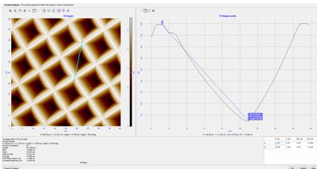
**Fig. 13. Determining the micro processing depth for the sample obtained with the M2 (10µm x 10µm) mask**
