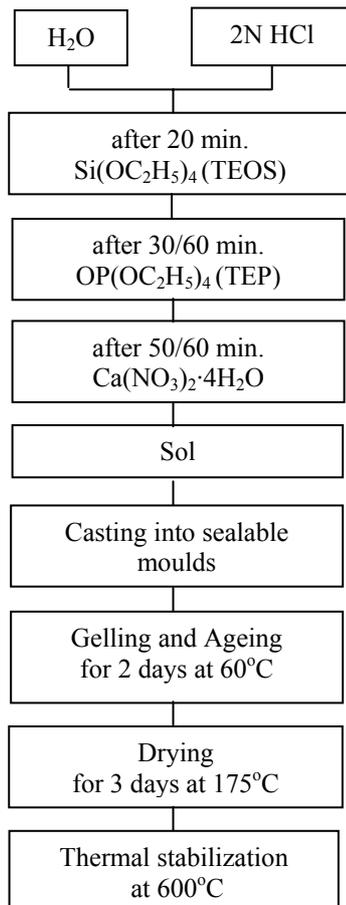
**Fig.2. Flow-chart for production of sol-gel glass powder**
