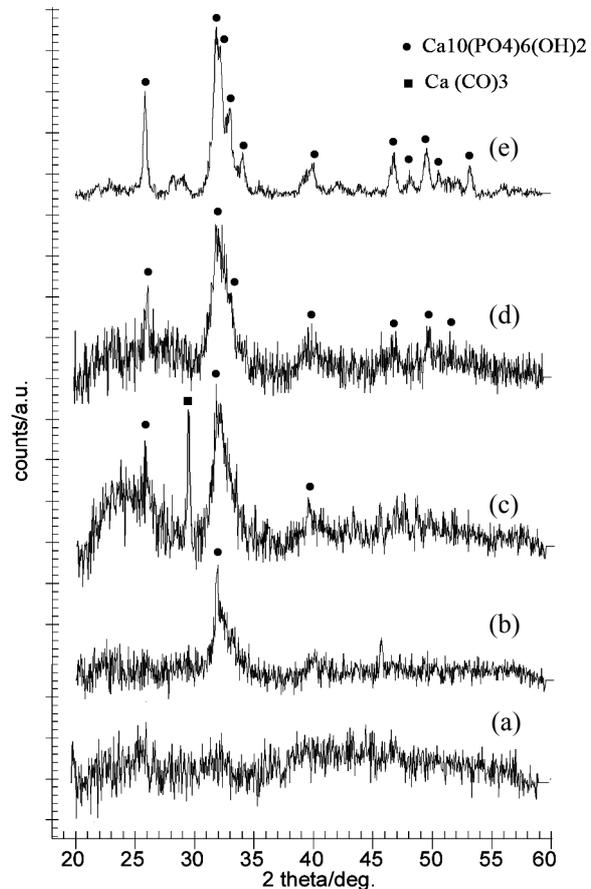
**Fig. 5. X – Ray diffraction patterns of S2 gel derived glass immersed in SBF from 0 to 14 days.**
