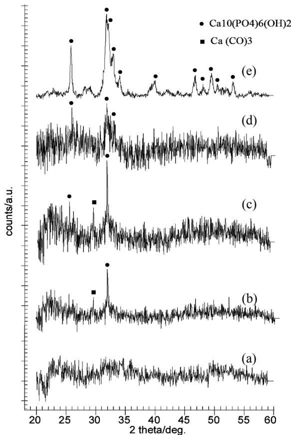
**Fig. 4. X – Ray diffraction patterns of S1 gel derived glass immersed in SBF from 0 to 14 days.**
