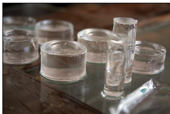
**Fig. 1. Gel samples in different shapes formed after keeping sol for about 60 hours in drying oven**
