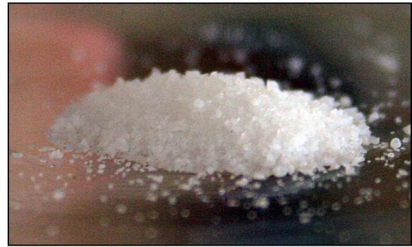
**Fig. 3. Sol-gel powder glass obtained after calcinations process**
